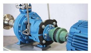
A size 7 TB Woods Sure-Flex Plus coupling was able to be installed instead of a larger size 8 coupling on this small ANSI pump unit. By utilizing the smaller coupling, the overall package length was reduced allowing for a smaller baseplate footprint.
