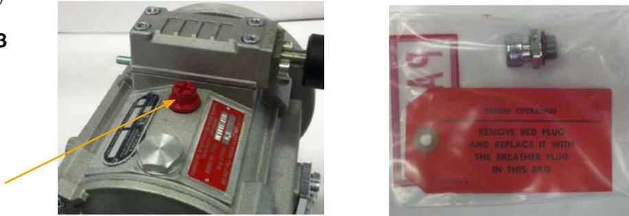
2. Before starting HSV, check the oil level at the sight port to make sure it is correct. Oil should be visible in sight port. (See arrow, Figure 4). If oil is not visible, add oil to proper level. Use the oil specification chart as a reference (Table 2).
