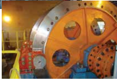
Svendborg brake for the high-speed side of a conveyor drive (above).
